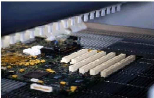
Fig 1: Board through Chemical Isolation Blow Off Section
